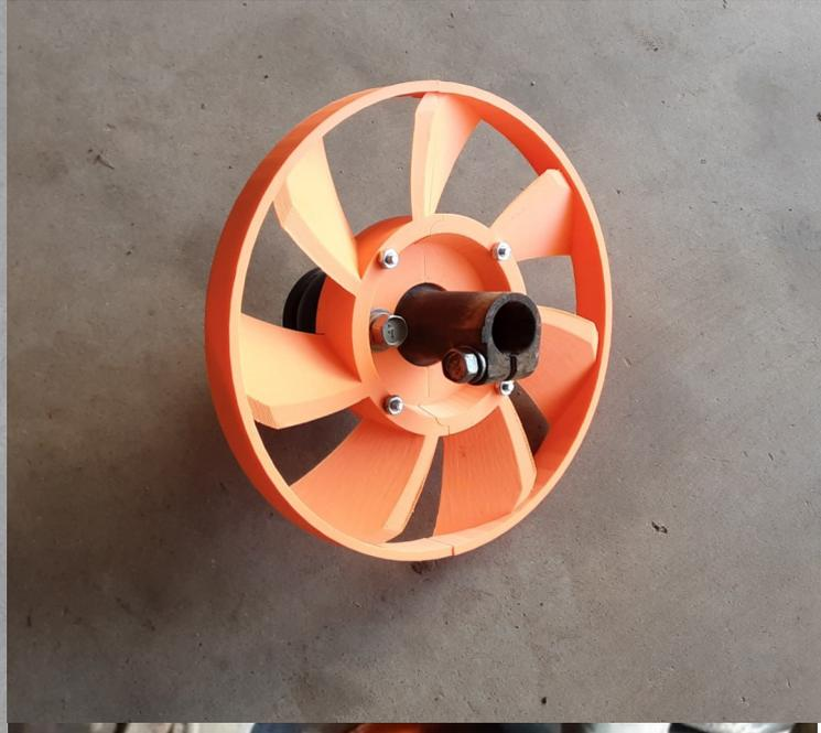
This orange HST fan fits all Kubota BX tractor models. This fan replaces the Kubota white hydraulic fan that is attached to the drive shaft, and is a direct replacement for Kubota part no K2561-14250 .
